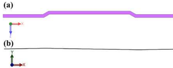
Fig. 2. Two different orientations of a Roebel strand detached from a Roebel cable. (a) Top view of a Roebel strand (b) Side view of a Roebel strand.
